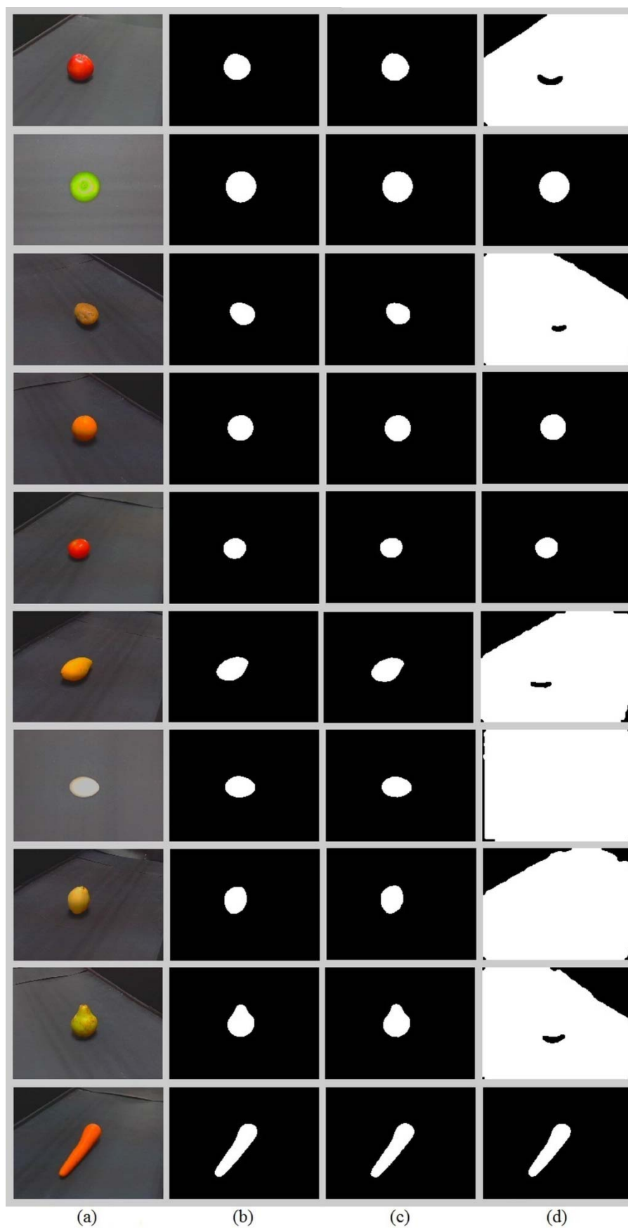
Fig. 6. (a) original image (b) proposed method (c) proposed by Siswantoro, et al. [18] (d) k -means clustering on the whole image
